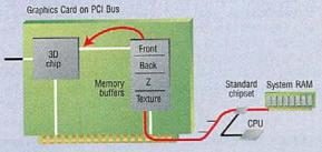
When present-day graphics cards run out of onboard memory, they store texture data in System RAM. When needed, data is copied to the card's local memory for processing.
